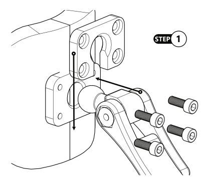
**STEP 1:** Place the 17mm ball in the socket located at the rear of the headrest. Slide the split ring over the shaft behind the ball and then towards the headrest to retain the ball.
