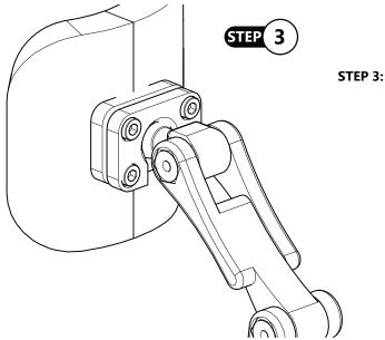
step 3: Working diagonally, evenly tighten the screws making sure the split ring remains parallel with the mount.
