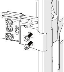
**Step Three:** Position the back post clamps at the proper height on the back post and tighten the M5x0.8x25mm Socket Head Screws to secure the mounting hardware to the back posts.
