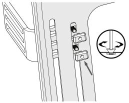
**Step Three:** Thread a Single Hole T-Nut (A7) onto each screw. Make sure the grooves in the T-nut line up with the edges of the slot. Lightly snug the screw to hold the mounting bracket in place.
