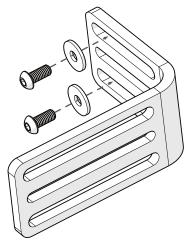
**Step Two:** Insert the screws and the mounting bracket into one of the mounting slots on the back shell.
