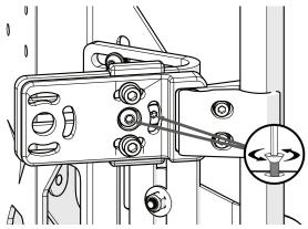
**Step Two:** Slide the back shell forward or backward to the desired depth. (**Note**: L-Brackets can be reversed to allow for more or less depth adjustment. This change affects width adjustability in a similar manner.)
