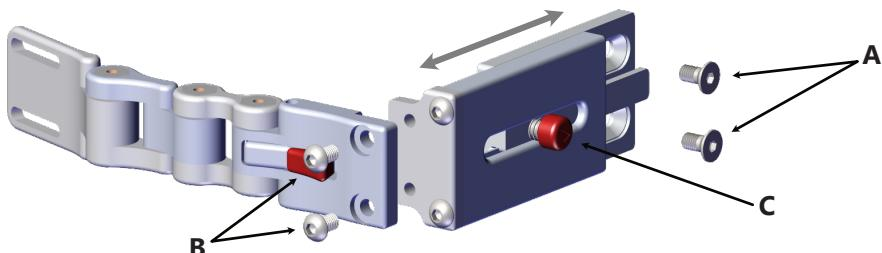
2. Use the M6 x 1.0 x 12mm Button Head Screws (B) to directly mount the lateral to the all-season bracket. Tighten with a 4mm Hex Wrench.
