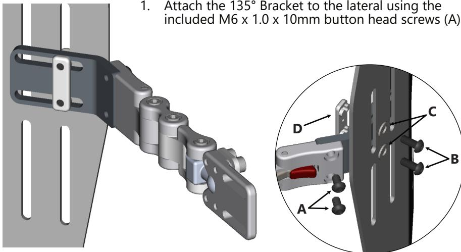
1. Attach the 135° Bracket to the lateral using the included M6 x 1.0 x 10mm button head screws (A).
