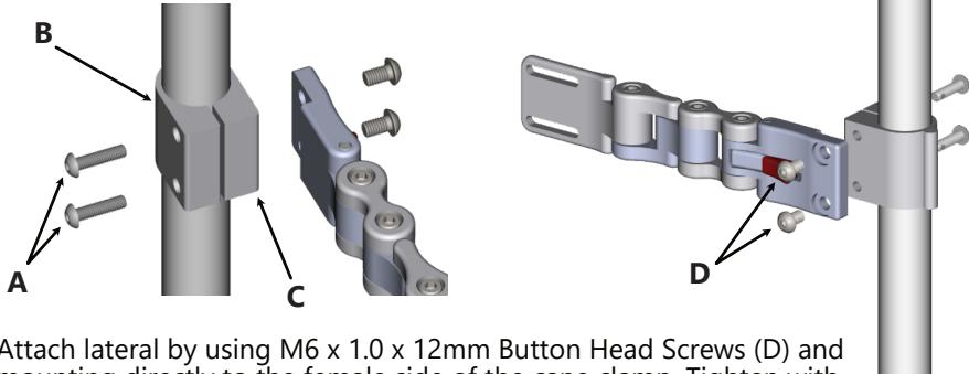
2. Attach lateral by using M6 x 1.0 x 12mm Button Head Screws (D) and mounting directly to the female side of the cane clamp. Tighten with an M4 Hex Wrench.
