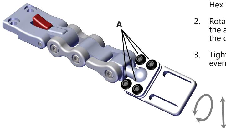
1. Loosen the M6 x 1.0 x 12mm Button Head Screws (A) with a 4mm Hex Wrench.
