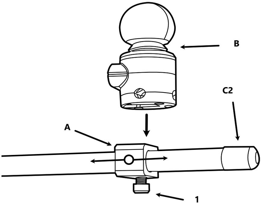
**Step Two:** Slide clamp (A) to desired horizontal position. Replace bar plug (C2). Hold clamping screw (1) and position Multi Joystick (B) in place over the clamp (A).
