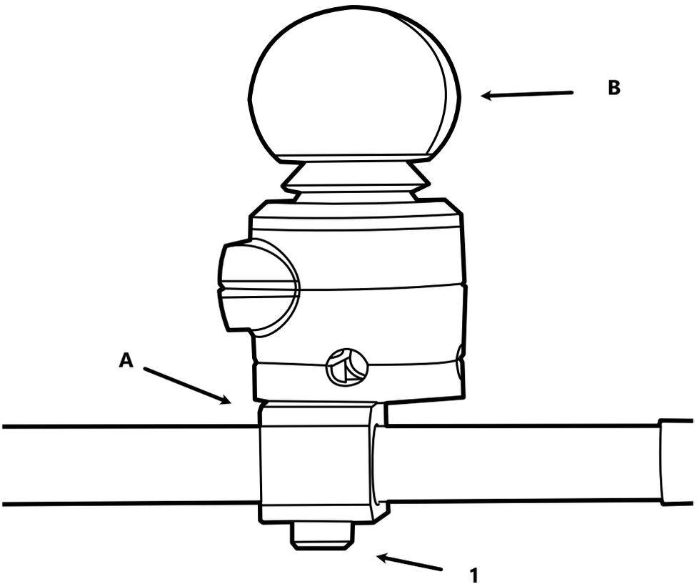
**Step Three:** Tighten the screw (1) with a 4mm hex key, taking care not to overtighten. Mount Multi Joystick (B) and tighten to clamp (A).
