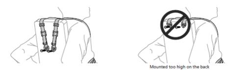
Fasten tri-ends to the seat back with the included fasteners and attach the belt to the tri-end. This will allow proper adjustment of the tension straps.
