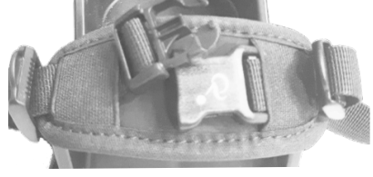
The side-release buckle is opened by pinching the buttons on it's sides until the halves separate. The ends are retained via elastic straps sewn to the pad.
