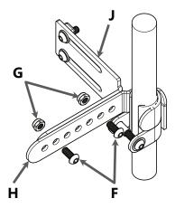
**Step Two:** To adjust the mounting hardware for depth, remove the two M6 x 1 x 16mm Button Head Screws (**F**) and M6 x 1 Nylon Lock Nuts (**G**) holding the 1 IN 7 Hole J-Hook (**H**) from the Double Slot Adjustable L-Bracket (**J**). Adjust the bracket to the desired holes and reinstall the screws to secure it in place.
