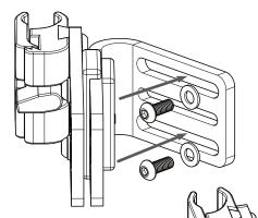
**Step One:** Place M6x1x16mm Button Head Screws (A5) and M6 Washers (A4) in the top and bottom slot of the Mounting Bracket\* (A).
