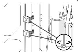
**Step Three:** Thread a Single Hole T-Nut (A7) onto each screw. Make sure the grooves in the T-nut line up with the edges of the slot. Lightly snug the screw to hold the mounting bracket in place.
