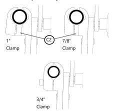
The All Purpose (Knob) Hardware is initially configured to fit a 3/4" cane. It can be adapted to fit a 1" cane and 7/8" cane with the large and small Tube Spacers (C2) as shown above.
