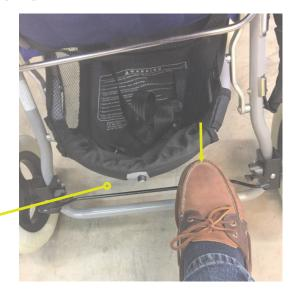
**Step Two:** To disengage the wheel lock, place your foot under the brake lever and, using your foot, pull the lever upwards. This will unlock both rear wheels.
