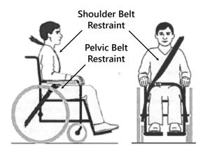
• Upper torso belt restraints should fit directly over, and in contact with, the middle of the shoulder.
