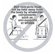
Belt restraints should not be routed outside of the wheelchair, over the wheelchair wheels, or over the wheelchair arm supports and should not be held away from the body by wheelchair components or parts.
