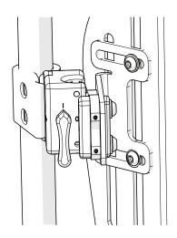
**Step Three:** Thread each screw into a Single Hole T-Nut (A4). Make sure the grooves in the T-nut line up with the edges of the slot. Tighten the screw to secure the mounting bracket in place.
