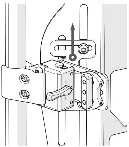
**Step Three:** To replace the back shell, slide the Latch Pin (B2) into the Back Post Clamps (C). Rotate the Cam Pin (C6) back to the vertical position to lock the back in place
