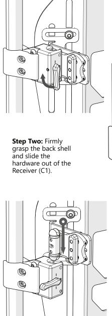
**Step One:** Rotate the Cam Pins (C6) a quarter turn on each removable hardware to unlock the mounting hardware from the Receiver (C1).
