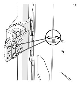
**Step Two:** Slide the Mounting Bracket (A) forward or backward into the desired position.
