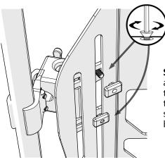
**Step One:** Place M6x1x12mm Button Head Screws (A2) and M6 Washers (A3) in the top and bottom slot of the Mounting Bracket\* (A1).
