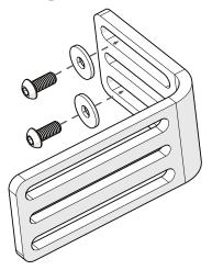
**Step One:** Place M6x1x16mm Button Head Screws (A5) and M6 Washers (A4) in the top and bottom slot of the Mounting Bracket (A)\*.
