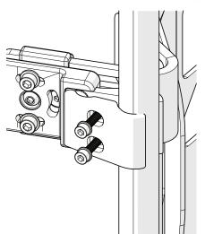
**Step Three:** Position the back post clamps at the proper height on the back post and tighten the M5x0.8x25mm Socket Head Screws to secure the mounting hardware to the back posts.
