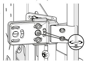
**Step Two:** Slide the back shell forward or backward to the desired depth. (**Note**: L-Brackets can be reversed to allow for more or less depth adjustment. This change affects width adjustability in a similar manner.)
