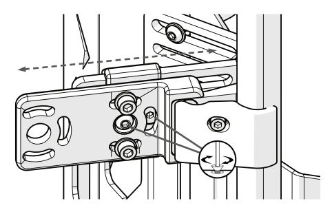
**Step Three:** Secure the back in the new position by tightening the M6x1x16mm Flat Head Screw (A6), the M6x1x20mm Button Head Screw (A8).
