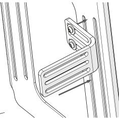
**Step Two:** Insert the screws and the mounting bracket into one of the mounting slots on the back shell.
