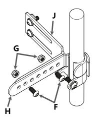
**Step Two:** To adjust the mounting hardware for depth, remove the two M6 x 1 x 16mm Button Head Screws (**F**) and M6 x 1 Nylon Lock Nuts (**G**) holding the 1 IN 7 Hole J-Hook (**H**) from the Double Slot Adjustable L-Bracket (**J**). Adjust the bracket to the desired holes and reinstall the screws to secure it in place.
