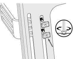
Step Three: Thread a Single Hole T-Nut (A7) onto each screw. Make sure the grooves in the T-nut line up with the edges of the slot. Lightly snug the screw to hold the mounting bracket in place.
