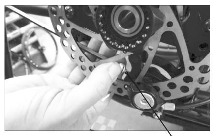
Further adjustment may be needed. See Caliper Adjustments section for instructions.
