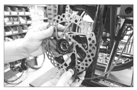
**Step 8:** Secure the rotor assemblies with the retaining rings provided.
