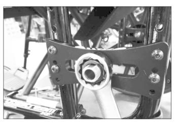
To ensure the proper location of installation, note the position of the axle receivers before removal.
