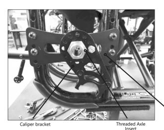
Position the caliper/caliper bracket and axle receiver assembly at an angle that gives the caliper ample room to operate and room for the cable to enter the caliper without too sharp of a bend.
