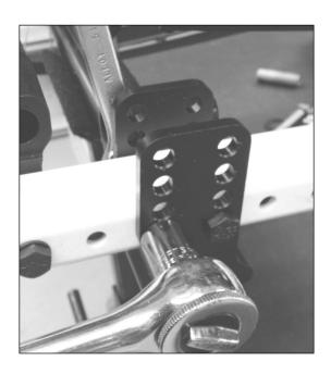
**Step 4:** Place the universal caliper brackets outside the OEM axle brackets and loosely install the 5/6" x 2.25 bolts supplied.
