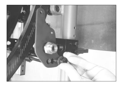
**Step 4:** Bolt the "U"-shaped caliper brackets to the tall brackets.
