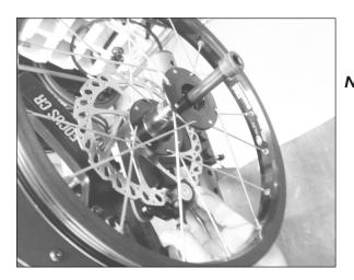
Note: Calipers are aligned to the rotor discs by the two silver caliper bolts opposite one another.
