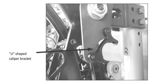
**Step 5:** Adjust the threaded axle receiver to the measurement shown for correct disc-to-caliper alignment, then tighten the corresponding lock nuts.
