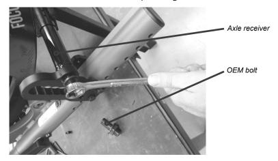
**Step 3:** Slide tall brackets into place. Loosely replace OEM hardware and axle receivers
