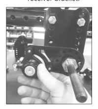
When deciding on an ideal caliper location, consider optimal brake cable routing and possible interference from the chair's tilting mechanism.
