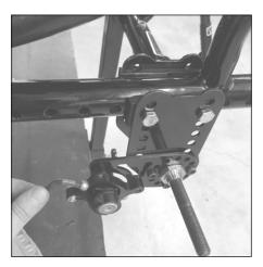
Step 7: Temporarily remove the caliper main body by removing the silver socket head screws on the caliper with a 5mm hex key.
