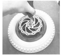
Step 9: Slide the removed caliper main body around the rotor and slide the wheel into position on the axle.
