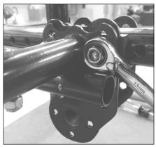
**Step 4:** Thread the large threads of the axle pin through the caliper bracket, then thread the bracket/axle pin back into the axle receiver bracket.
