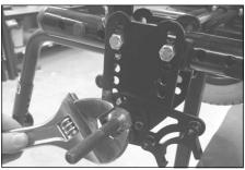
Step 6: With the caliper bracket now secured to the axle bracket, fully tighten the axle into the axle bracket.
