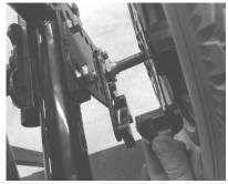
**Step 10:** Use a 3/4" socket or wrench to tighten the wheel with the lock nut.
