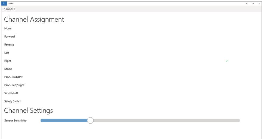
After having selected a particular channel, a screen will pop up listing the available selections for that channel, along with an adjustment bar for the input sensor sensitivity.
