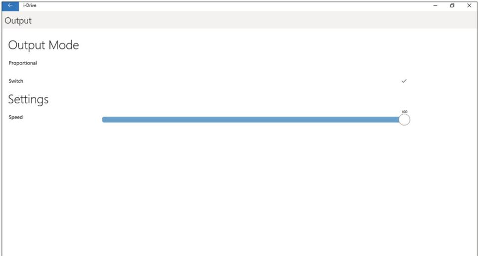
Selecting 'Output' allows a user to change the i-Drive's output mode from proportional to switched, or vice-versa. It also allows a user to adjust the output speed.
