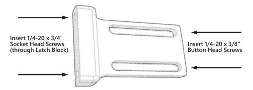
**Step One:** Attach the planar mount to the lateral latch block by inserting the two (2)  $1/4-20 \times 3/4$ " socket head screws through the face of the latch block and into the planar mount. (The planar mount and the lateral latch block will be joined at a 90° angle.)
