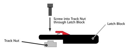
**Step One:** Loosely attach the track nut to the lateral latch block by inserting the two socket head screws provided through the face of the latch block and into the track nut as pictured above.
