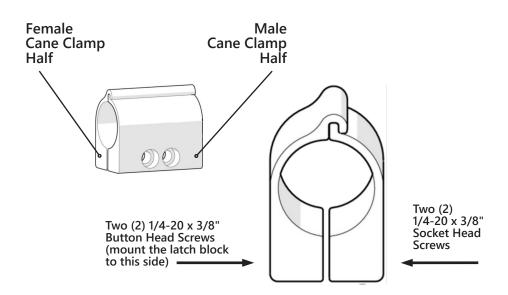
**Step One:** Identify the male cane clamp half and the female cane clamp half.
