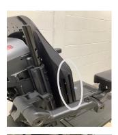
**2.** Slide the angled 125° lateral mounting bracket in behind the square plate in the lateral cover slot.
