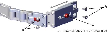
Use the M6 x 1.0 x 12mm Button Head Screws (B) to directly mount the lateral to the all-season bracket. Tighten with an M4 Hex Wrench.
