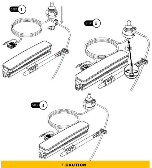
Ensure that all screws are tightened evenly on the hardware. Threads can strip out and cause damage to the hardware if not tightened properly.
