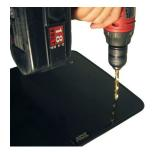
9. Drill four 3/16in. holes where the seat base is marked.
