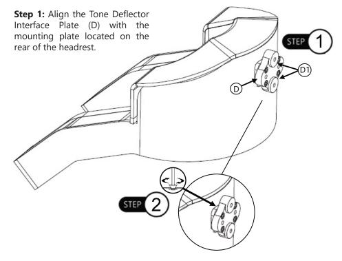
**Step 2:** Insert and thread the four (4) M5x0.8x10mm Socket Head Screws\* (D1) through the interface plate and into the holes in the mounting plate of the headrest. Tighten evenly with a hex key.
