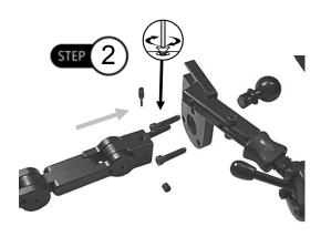
**Step 3:** After the CPS9 Ring is mounted to the hardware, with a 5/32" hex tool fasten the socket head screws into the adjacent holes on the CPS9 and Comfort Plus Headrest.
