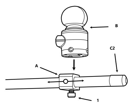
**Step Two:** Slide clamp (A) to desired horizontal position. Replace bar plug (C2). Hold clamping screw (1) and position Multi Joystick (B) in place over the clamp (A).
