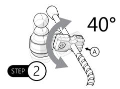
**Step 2:** Rotate block (A) in a 40° range to desired height. Tighten screws again.
