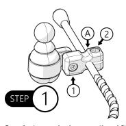
**Step 1:** Loosen both screws (1 and 2).
