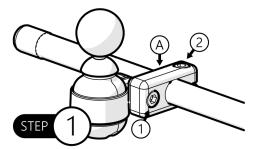
Step 1: Loosen both screws (1 and 2).
