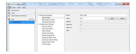
Clicking on the Reset Button will set the parameter value back to the default value. Click Apply to store locally and Save to make the change to the device.
