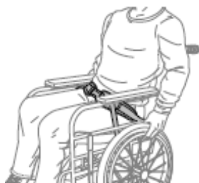
4-Point hip belt over the ASIS with main webbing running parallel to seat surface.
