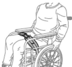
2-Point hip belt in position over the upper thigh, pulling downwards and backwards.
