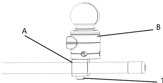
**Step Three:** Tighten the screw (1) with a 4mm hex key, taking care not to over-tighten. Mount clamp (A) and tighten to Multi Joystick (B).
