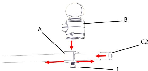
**Step Two:** Slide clamp (A) to desired horizontal position. Replace bar plug (C2). Hold clamping screw (1) and position Multi Joystick (B) in place over the clamp (A).
