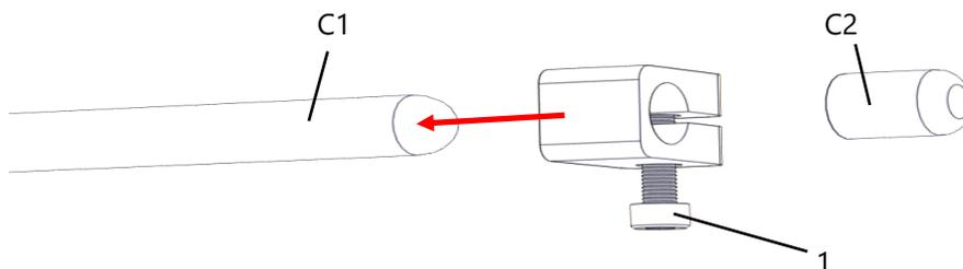
**Step One:** Remove bar plug (C2) from Gatlin arm (C1). Loosen clamping screw (1). Slide clamp (A) onto the arm (C1).
