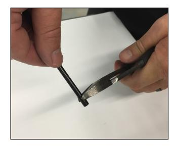
**Step 7:** Run one end of the cable through the lower hole in the lever, pulling the cable until the MTB brad fits securely in the recess.
