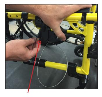
**Step 9:** Feed the cable through the cable housing, checking for smooth operation.
