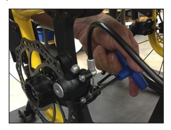
Step 12: Cut away any excess cable, approximately 6" to 1'.
