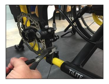
**Step 12:** Cap and crimp the cable ends to prevent wear/unraveling.
