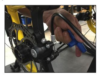
**Step 11:** Cut away any excess cable, approximately 6" to 1'.
