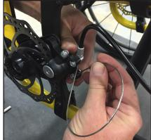
**Step 11:** Pull to remove all slack from the cable; tighten clamp screws with a 4mm hex key.
