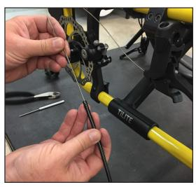
**Step 10:** Run the cable through the caliper's cable input ferrule and down through the slot on the caliper's clamping arm, ensuring the cable housing is fully seated in the cable input ferrule.
