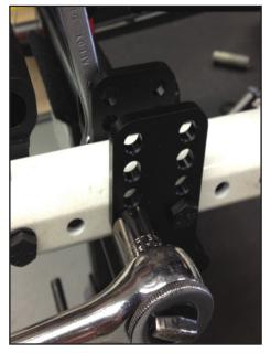
**Step 4:** Place the universal caliper brackets outside the OEM axle brackets and loosely install the  $5/16" \times 2.25$  bolts supplied.
