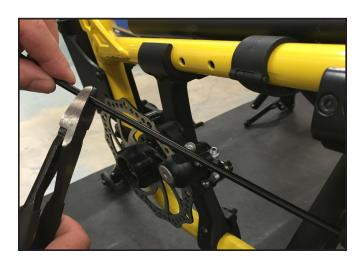
**Step 6:** Gently crimp a metal end cap to both ends of the cable housing.
