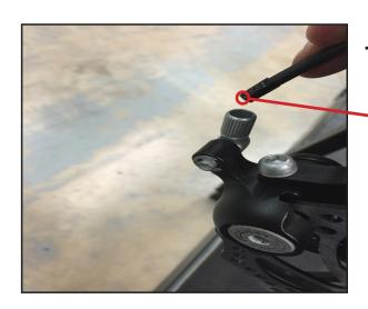
To gauge the necessary length of housing, gently crimp a metal end cap to one end of the housing and insert this crimped end into the cable input ferrule on the caliper. Then route the housing to the lever input and mark the length to ensure a clean, clear housing cut.
