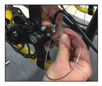
**Step 10:** Pull to remove all slack from the cable; tighten clamp screws with a 4mm hex key.
