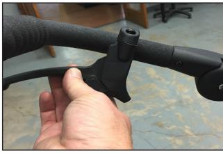
**Step 2:** Determine the desired mounting locations for the levers. Use box cutters to cut away any obstructive padding or grips and ensure space for the lever handle.
