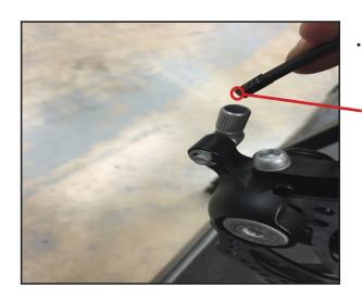
To gauge the necessary length of housing, gently crimp a metal end cap to one end of the housing and insert this crimped end into the cable input ferrule on the caliper. Then route the housing to the lever input and mark the length to ensure a clean, clear housing cut.
