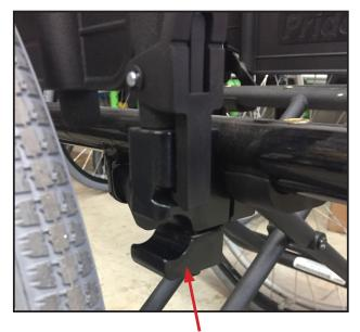
**Step 2:** Insert the lever adjustment bar into the existing frame clamp; adjust position as necessary.
