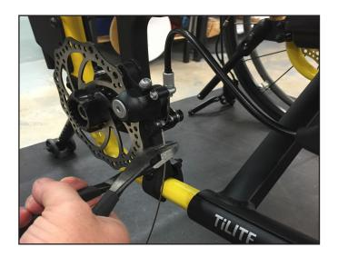
**Step 13:** Using end caps provided, cap off and crimp the cable ends to prevent wear/unraveling.
