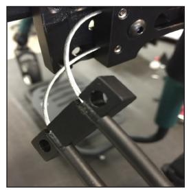
**7c)** Secure the housing clamp screws with a 3/32" hex key.
