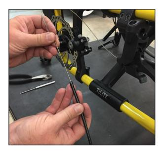
**Step 9:** Run the cable through the caliper's cable input ferrule and down through the slot on the caliper's clamping arm, ensuring the cable housing is fully seated in the cable input ferrule.
