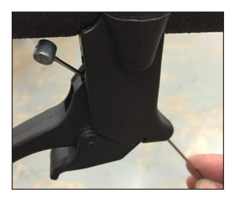
**Step 8:** Feed the cable through the housing, checking for smooth operation.
