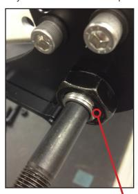
**Step 7:** Once the axle is tight, the 5/16" x 2.25 bolts can be tightened.
