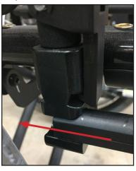
**Step 3:** When the lever adjustment bar is in the desired position, use a hex key to tighten the screws on the frame clamp.
