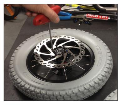
**Step 9:** Place the wheel assemblies over the axles, spinning the wheels to check for any interference. Adjust spindles accordingly. Use the 1/2"-20 lock nuts provided to secure the wheels.
