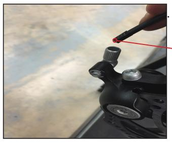
To gauge the necessary length of housing, gently crimp a metal end cap to one end of the housing and insert this crimped end into the adjustable cable input ferrule on the caliper. (Do this with both the same-side and the opposite-side calipers, ensuring equal cable length on both sides.)
