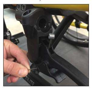
**Step 8:** Guide the cable through the lever's housing slot.
