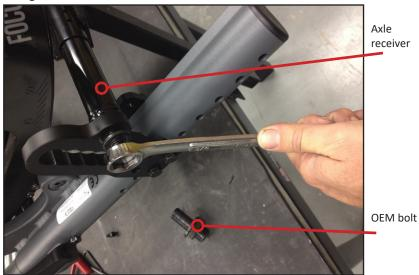
**Step 3:** Slide tall brackets into place; loosely replace OEM hardware and axle receivers.
