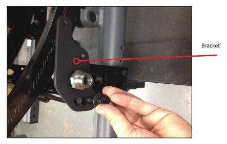
**Step 4:** Bolt the "U"-shaped caliper brackets to the tall brackets.
