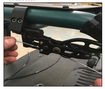
**6b)** When the cables are fully seated, use a 3/32" hex key to tighten the set screws on the cable block.
