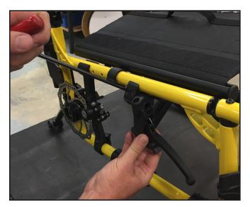
**Step 4:** Determine the amount of cable/housing necessary to attach the lever to the cable input ferrule on the caliper.
