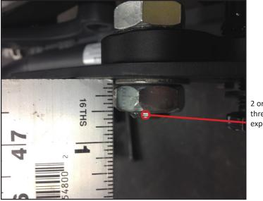
2 or 3 threads exposed Step 6: Tighten the OEM bolt.
