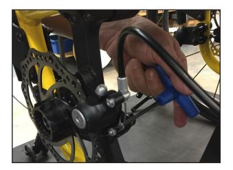
Step 11: Cut away any excess cable, approximately 6" to 1'.
