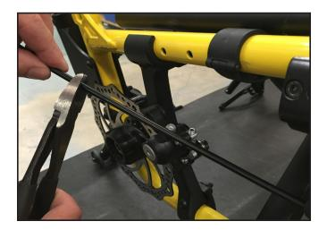
**Step 6:** Gently crimp a metal end cap to both ends of the cable housing.
