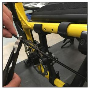
**Step 6:** Gently crimp a metal end cap to both ends of the housing.
