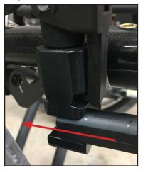
**Step 3:** When the lever adjustment bar is in the desired position, use a hex key to tighten the screws on the frame clamp.
