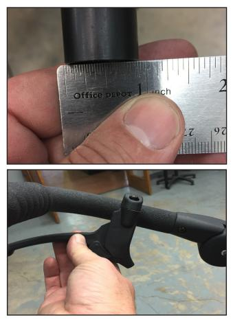
**Step 2:** Determine the desired mounting locations for the levers. Use a box cutter to cut away any obstructive padding or grips and ensure space for the lever handle.
