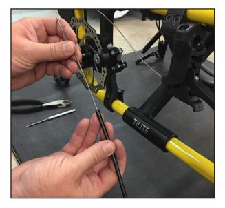
**Step 9:** Run the cable through the caliper's cable input ferrule and down through the slot on the caliper's clamping arm, ensuring the cable housing is fully seated in the cable input ferrule.
