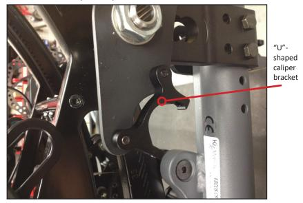
Step 4: Bolt the "U"-shaped caliper brackets to the tall brackets.
