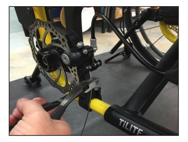
Step 12: Cap and crimp the cable ends to prevent wear/unraveling.
