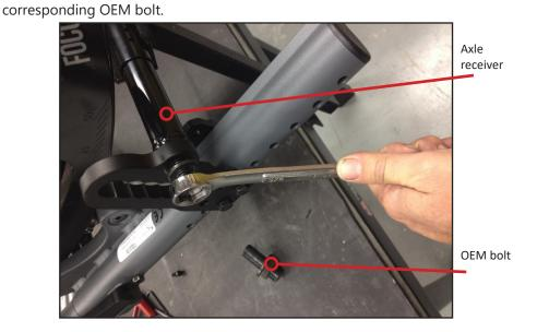
Step 2: Working one side at a time, remove each threaded axle receiver and each
