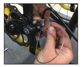
**Step 10:** Pull to remove all slack from the cable; tighten clamp screws with a 4mm hex key.
