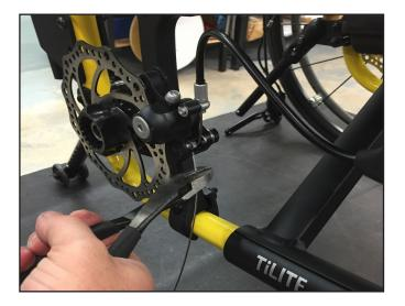
**Step 13:** Using end caps provided, cap off and crimp the cable ends to prevent wear/unraveling.
