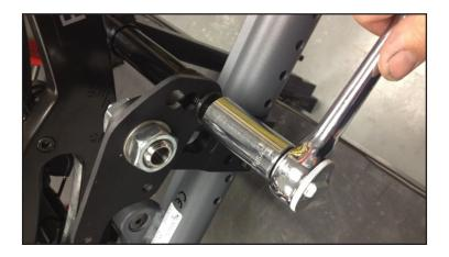
Step 7: Using the Torx cap screws provided, bolt the rotor discs to the wheels.
