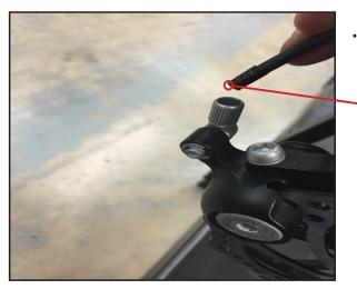
To gauge the necessary length of housing, gently crimp a metal end cap to one end of the housing and insert this crimped end into the cable input ferrule on the caliper. Then route the housing to the lever input and mark the length to ensure a clean, clear housing cut. **Step 5:** Cut a length of housing, ensuring the cuts are clean and free of obstructions that may drag on the cable.
