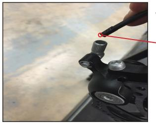
To gauge the necessary length of housing, gently crimp a metal end cap to one end of the housing and insert this crimped end into the cable input ferrule on the caliper. Then route the housing to the lever input and mark the length to ensure a clean, clear housing cut. **Step 5:** Cut a length of cable housing, ensuring the cuts are clean and free of obstructions that may drag on the cable.
