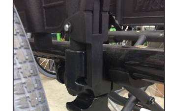
• It is recommended that after the lever is mounted, it should not extend past the chair's frame when engaged fully forward.
