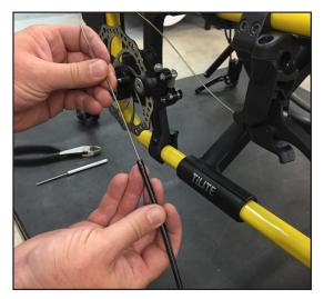
**Step 10:** Run the cable through the caliper's cable input ferrule and down through the slot on the caliper's clamping arm, ensuring the cable housing is fully seated in the cable input ferrule.
