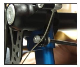
**9b)** Use a 4mm hex key to tighten the caliper clamp screw, locking the cable to the clamps.
