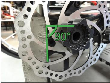
**Step 9:** Use a 3/16" hex key to tighten the chair's camber tube clamps and lock this position.
