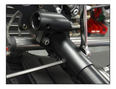
**Step 8:** Using a builder's square, rotate the camber tube so the vertical, flat surfaces of the camber tube weldment are at a 90° angle to the floor and the back column of the builder's square, and are at ride height. This sets proper "toein, toe-out" positioning.
