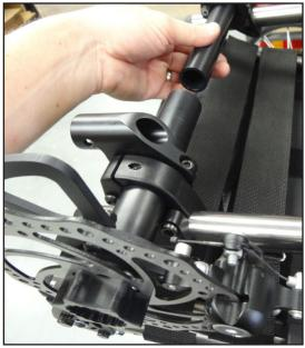
**Step 5:** Beginning rearward, loosely install two 6mm x 35 bolts through the camber tube ends and the center tube slots, with two 6mm locking nuts toward the front of the assembly.
