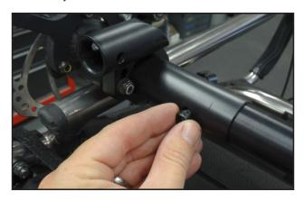
**Step 6:** Using wheels with spline drives installed, position each disc brake assembly according to the specifications noted from the measurements taken in Step 1.
