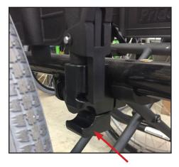
**Step 2:** Insert the lever adjustment bar into the existing frame clamp; adjust position as necessary.
