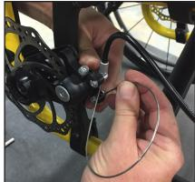
**Step 11:** Pull to remove all slack from the cable; tighten clamp screws with a 4mm hex key.
